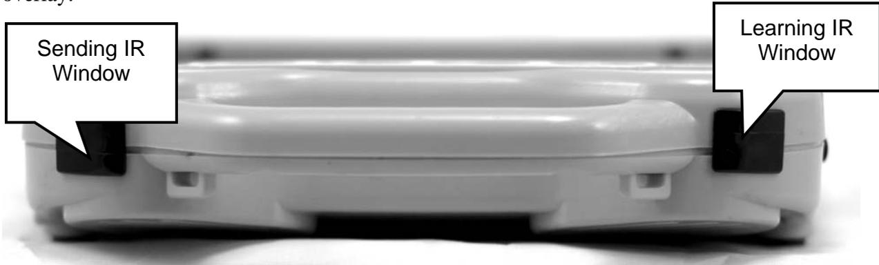
The IR windows are on the top of your SpringBoard. They are the black windows on either side of the handle. If you want to **teach** the SpringBoard a signal, you point your remote control at the window on the right as shown in the picture above. If you want the **send** a signal that the SpringBoard has learned, make sure the top of the device is facing in the general direction of the appliance you want to send the signal to.
