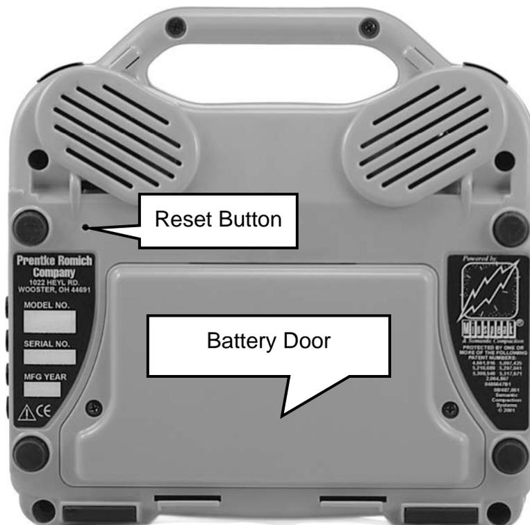
**Battery Door:** The device batteries are underneath this door. There is also a card slot at the top of the battery door that holds the system software card. Should you need to, you can remove the battery door by unscrewing it from the case.
