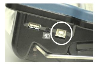
Connect the small square plug at one end of the USB cable to the square USB port on the left side your Pathfinder.
