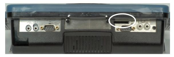
The Secure Digital card is already in place in its slot on the top of the Pathfinder.
