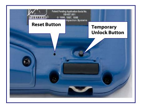
**Reset Button** Unbend a paper clip and poke it into the hole to
